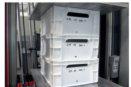
Fig. 3. Stacking pressure test with three stacked transport boxes with sandwich structure. Top: without pressure loading; bottom: strong pressure loading on the boxes visibly leads to a compression of the side walls and reinforcing ribs © TCKT – Transfercenter für Kunststofftechnik GmbH
